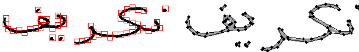
Figure 5.8 Division of a word into sub-images and its polygon approximation
