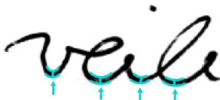
Figure 2.9 Segmentation into fraglets (Image: [Schomaker et al., 2004])
