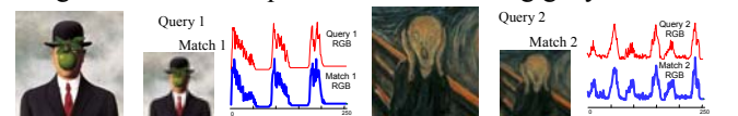
Figure 12. left ) A detail of The Son of Man by René Magritte, which we used as a query to our index, finding “Match 1”. right ) A detail of The Scream by Edvard Munch, which we used as a query that returned “Match 2”. The insets show the similarity of the images in RGB histogram space.
