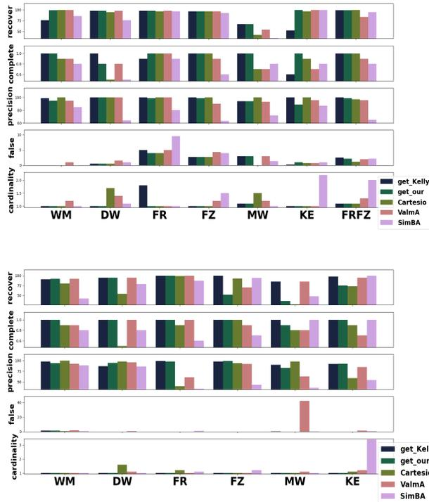
Figure 14: Accuracy comparison of activations extraction for REFIT (above) and UK-DALE (below)
