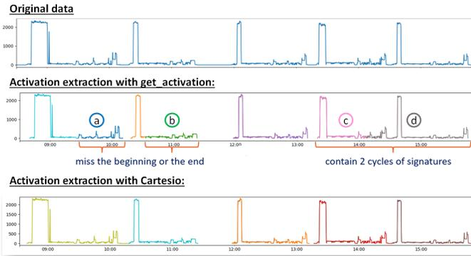
**Figure 3: Example of activations extraction for the get\_activations method and Cartesio. At the top the original data. In the middle results from get\_activations: a&b) omission of the beginning of the activation sequence; c) omission of the end of the activation sequence; d) get\_activations considers two neighboring activations as a single activation. At the bottom, results of Cartesio: Cartesio correctly identifies all activations.**
