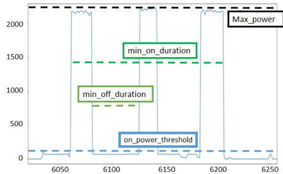
**Figure 1: Illustration of Kelly `get_activations` method. We keep activations whose power are more than `on_power_threshold` and less than `max_power`. Activation also needs to last more than `min_on_duration` and with interwindow duration shorter than `min_off_duration`.**
