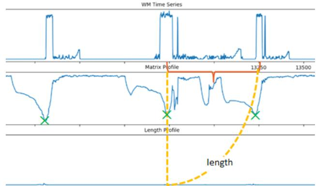
**Figure 6: ValmA: How to extract activations from the original results. The yellow line delimits the signature length. The green crosses indicate the beginning of a new activation.**
