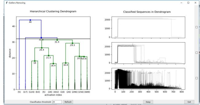
Figure 8: GUI that allows the user to select barycenters (washing machine example)
