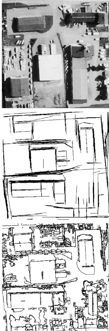
Fig. 3. Two partial gestalts, alignments and boundaries. Top: original aerial view (source: INRIA), middle: maximal meaningful alignments, bottom: maximal meaningful boundaries.
